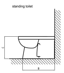
According below drawings, it should be ensured that from the toilet bowl center axle left and right at least 350 mm free space available, to be able to use the stand support.
